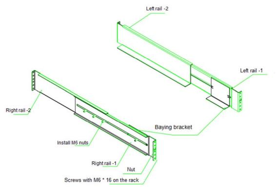
As shown in the above figure, assemble the left rail, right rail, baying bracket and nuts, then install the slide rails into the rack. You can adjust the depth to match the rack by the slide rails. The rail can be compatible with a minimum of 440 mm, and a maximum of 711 mm.
