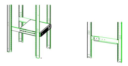
Adjust the rail according to depth of the rack. It should not be greater than the maximum size of the rack rail, and not be shorter than the minimum size of the rack rail as well. Fasten the rails with screws.
